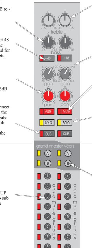
The TREBLE controls give continuous adjustment of boost and cut from +15dB to -15dB with a 0dB centre detent. The frequency is fixed at 10KHz.
