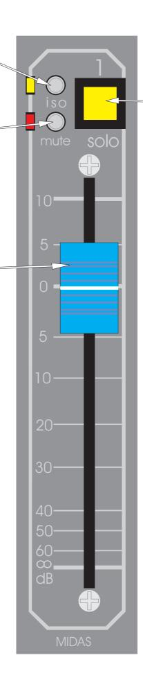
The vca SOLO switches are used to monitor VCA sub groups by creating a corresponding AUDIO sub group on the stereo AFL busses. All input channels and line returns that are assigned to a specific vca sub group will be summed onto the solo busses when that vca solo is active.
