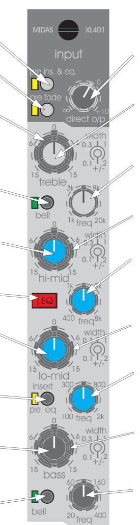
The DIRECT output control gives continuous adjustment of the direct output level from + 10dB to off. The output is derived from the input channel post fader signal.
