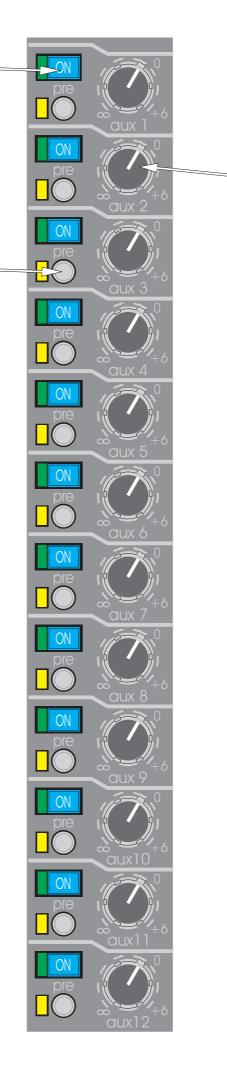
The mono AUX controls (1 to 16) give continuous adjustment of the level sent from the input channel to the aux busses. The signal is a mono sum of the left and right signals and the level adjustment is from + 6dB to off. The stereo aux ON switches connect signals from the input channel to the stereo aux busses and are under automation control.
