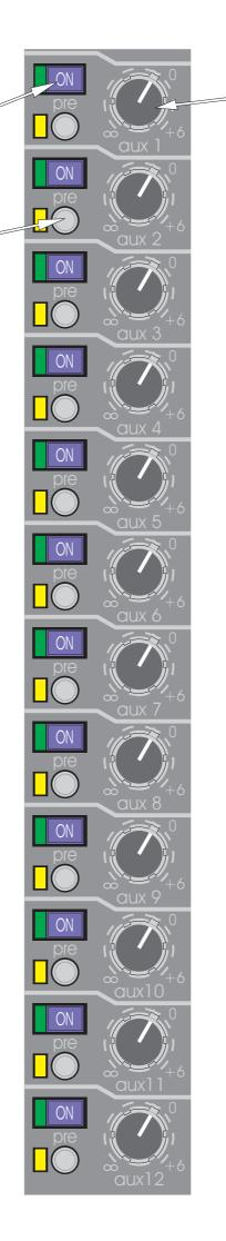
The mono AUX controls (1 to 16) give continuous adjustment of the level sent from the input channel to the aux busses. The level adjustment is from + 6dB to off.
