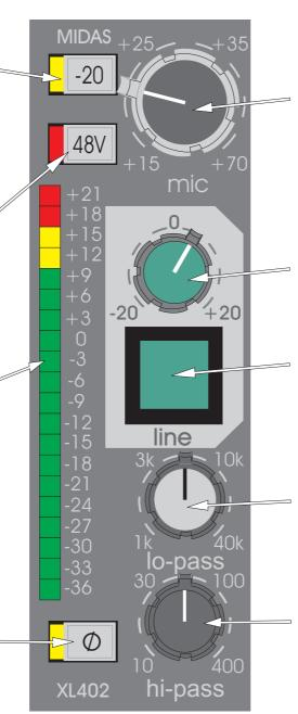
The MIC control gives continuous adjustment of the mic amp gain from + 15dB to + 70dB.
