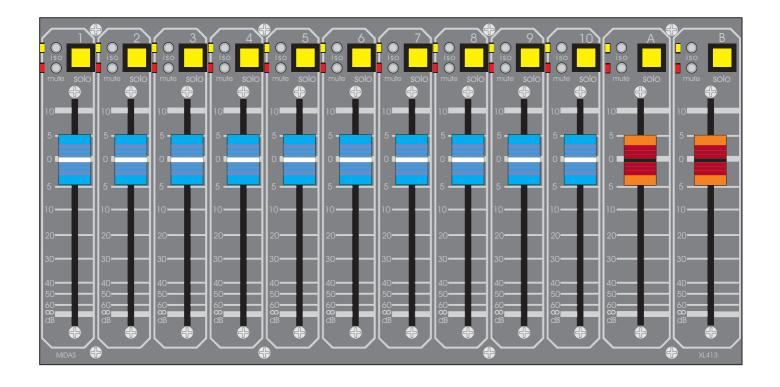
FUNCTION: Moving fader control of 10 VCA sub groups and 2 grand masters with facility to meter and solo listen.
