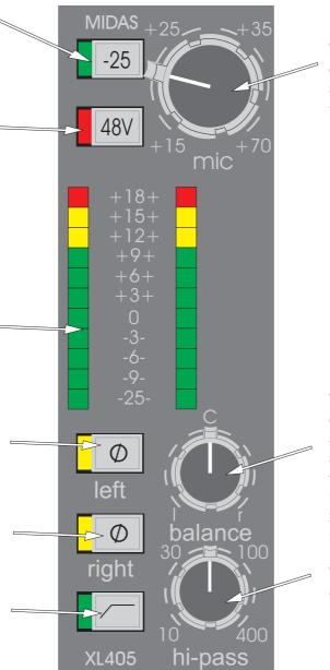
The MIC control gives continuous adjustment of left and right mic amp gains from +15dB to +70dB.
