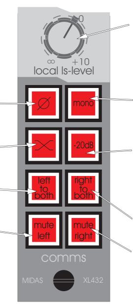
The LOCAL LS LEVEL control gives continuous adjustment of signals sent to the "A" or "B" monitor speaker outputs and has a range from + 10dB to off.
