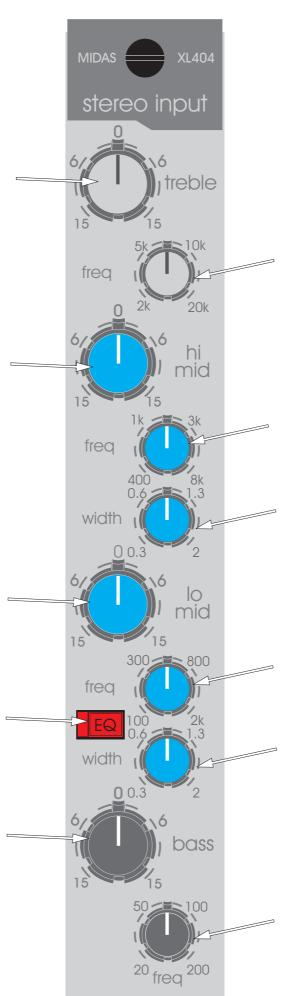
The treble FREQ control gives continuous adjustment of the frequency range that the treble equalisers act on from 2K to 20K.
