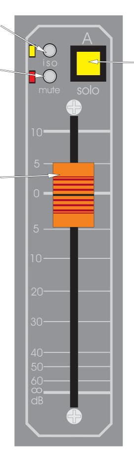
The grand master A and B vca SOLO switches are used to monitor the grand master A and B VCA sub groups by creating a corresponding AUDIO sub groups on the stereo AFL busses. All AUDIO sub groups that are assigned to grand master vca A or B will be summed onto the solo busses when the vca solo is active.
