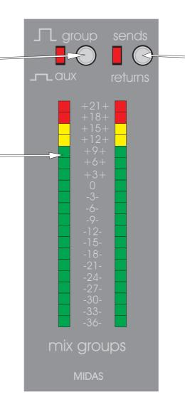
The RETURN switch changes the function of the left and right meters so that they monitor the post fader line return signals. If the AUX switch is not activated the meters return to monitoring the audio group outputs regardless of the RETURN switch position.
