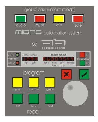
The top four switches, labelled 'AUDIO', 'MUTE', 'VCA' & 'LOCK' are not directly part of the central control CPU, these switches directly control the operating mode of the input fader automation. (See Input fader mode control, later).
