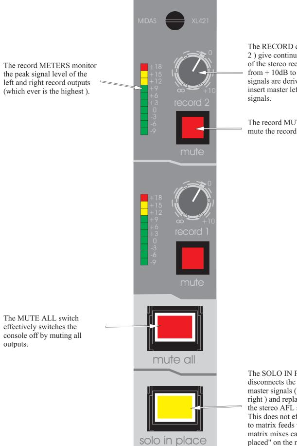
The RECORD controls (1 and 2) give continuous adjustment of the stereo record outputs from + 10dB to off. The record signals are derived from the pre insert master left and right
