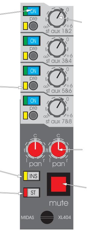
The ST AUX controls (1 to 8) give continuous adjustment of the level sent from the input channel (post pan) to the stereo aux busses. The level adjustment is from + 6dB to off.
