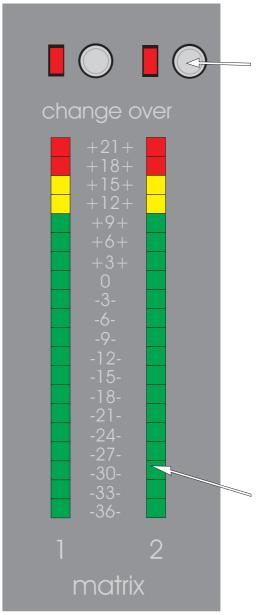
The CHANGE OVER switches change the function of the left and right meters so that they monitor the stereo aux send outputs in place of the matrix outputs.
