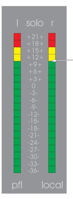
The meters monitor the peak signal level of the stereo AFL left and right solo busses or the PFL and local output level. The change over is automatic as part of the PFL Monitor switch on the COMMS module.
