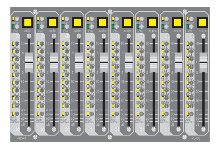
FUNCTION: Fader control of 48 input levels to stereo bus, audio sub groups and VCA sub groups with solo and mute group assign.
