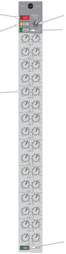
The STEREO AUX MASTER control gives continuous adjustment of the stereo aux output level from + 10dB to off.
