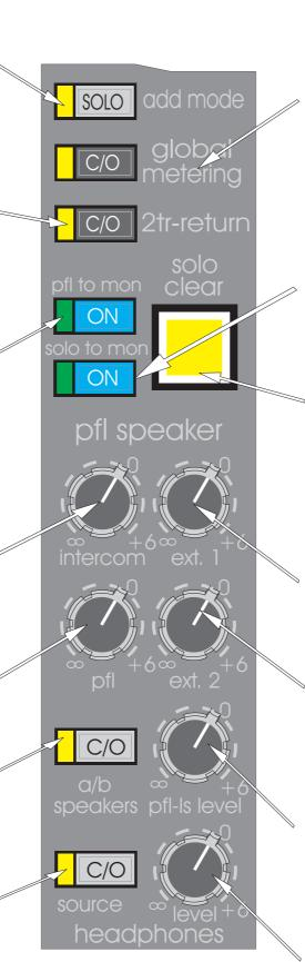
The GLOBAL METER CHANGE OVER switch changes the operation of every meter on the console except the comms meters and the record meters. The "normal" meter operation is to monitor pre fader on input channels and post fader on all other signals. When the global meter change over is active the meters change to monitor input amplifiers or bus amplifiers (as appropriate) on all signals.
