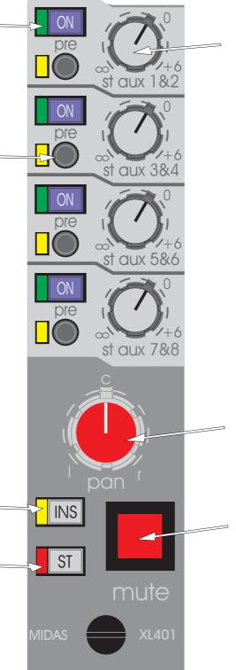
The ST AUX controls (1 to 8) give continuous adjustment of the level sent from the input channel (post pan) to the stereo aux busses. The level adjustment is from + 6dB to off.
