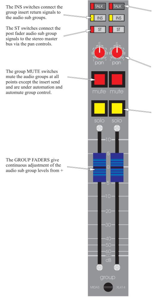
The TALK switches connect the audio sub groups to the COMMS module. When the TALK TO GROUPS switch on the COMMS module is activated it is then able to route its oscillator, pink noise, external input, talk mic or comms mic to the audio sub groups.
