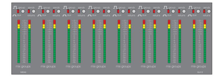
FUNCTION: To meter 16 group outputs, 16 aux master sends and 16 line level returns.
