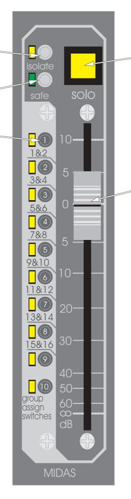
The SOLO switch sends the input channel signal to the PFL mono and AFL stereo busses. If the switch is pressed for a short time it will latch on or off, but, if it is held on for more than 1 second the latching is disabled and when the switch is released the channel solo will turn off.
